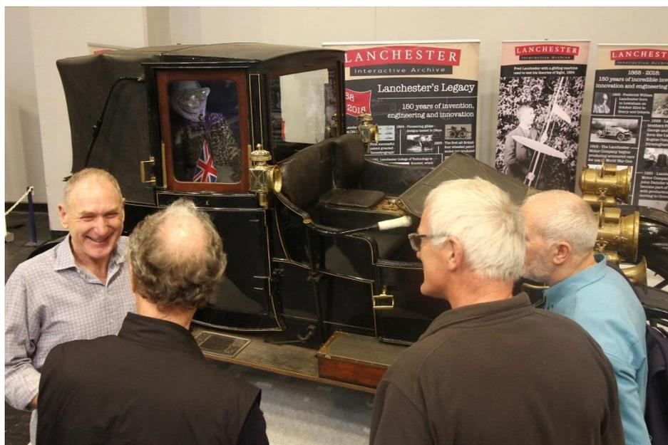
This was a 113-year-old 20hp Lanchester, currently under restoration, which hasn't been on the road since 1950. With the between-the-seats engine and gearbox removed, a flat floor was temporarily installed so that visitors could step easily across the car to sit in either front seat, behind the leather, folding dashboard.
