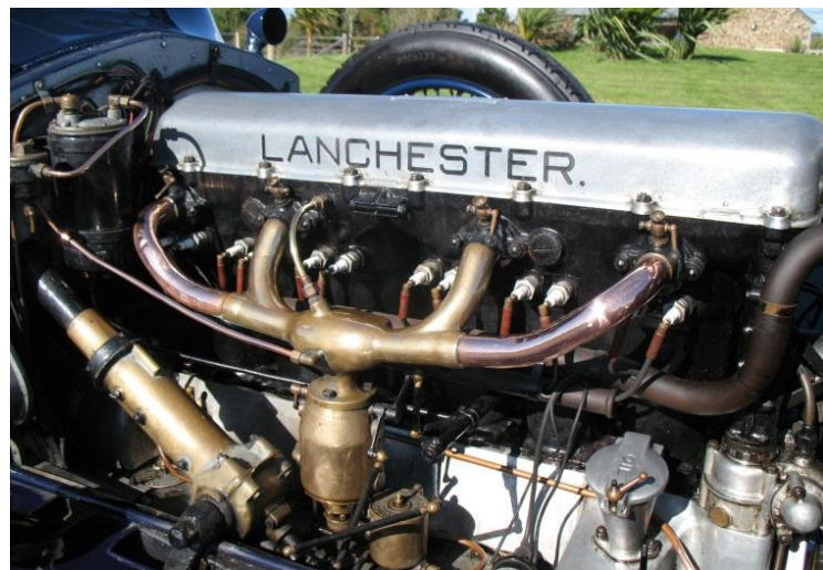
Figure 5. Offside view of engine with its magnificent inlet manifold
